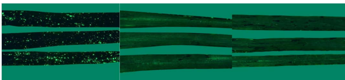
Figure 7: Comparison of GF-3308 (i-Q4) applied at 100 L/ha, 12 km/h, with 3-Star (75% DR Teejet TTI 025) and '4-Star' (90% DR Lechler ID3-05) nozzle, 3.0 and 2.0 bar Water 90% DR, Lechler ID3 05 i-Q4, 75% DR, Teejet TTI 025 i-Q4 90% DR, Lechler ID3 05
